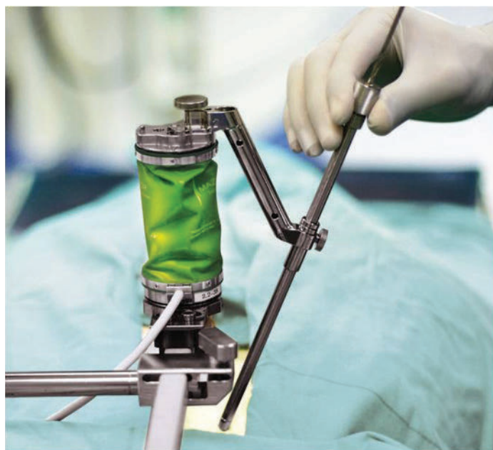
Figure 13. The Mazor Robot is attached to the spine of the patient and the arm is helping to guide the surgeon's hand during a minimally invasive surgery. Image courtesy Mazor Robotics, Ltd.
