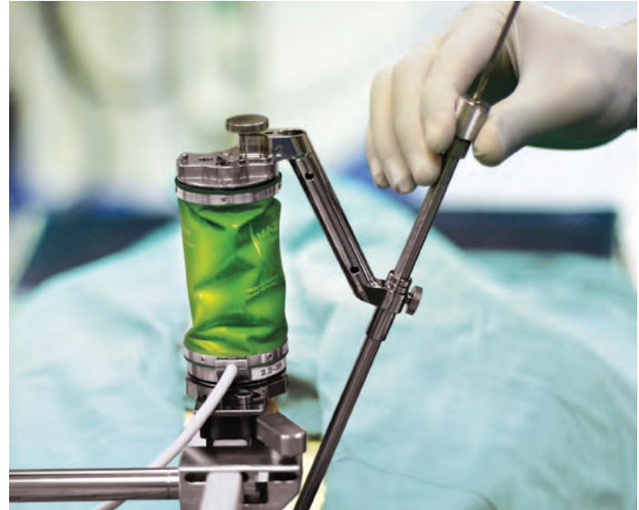
Figure 2. The Mazor Robot is attached to the spine of the patient. The robot arm helps guide the surgeon's hand during a minimally invasive surgery. Image courtesy of Mazor Robotics.
