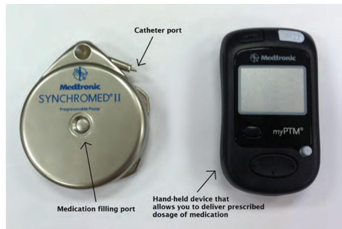
Figure 7. This intrathecal pain pump is implanted under the skin of the abdomen and delivers pain medication directly to the spinal cord.
