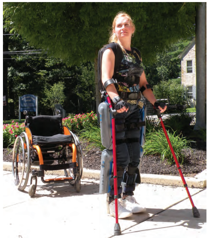
The ReWalk suit enables ambulation for those with thoracic level motor complete spinal cord injury. Image courtesy of Argo Medical Technologies.
