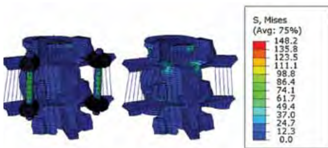
Figure 12: The figure above shows Von Mises stress (in MPa) contours of a validated L4-L5 spinal model with rigid (titanium) posterior instrumentation (left) and intact (right), for extension of 7.5Nm with 400N of follower load. The stress shielding of neural arch is seen in the case of posterior instrumentation (left) while intact (right) shows normal stresses on the neural arch.
