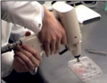
Figure 6. A gene gun being used to transfer genetic material into cells in the lab (Courtesy of Medical Research Council)
